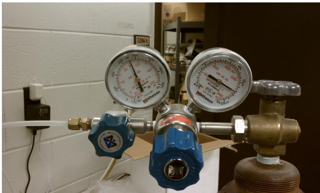
Figure B.4. Pressure regulator for argon tank
