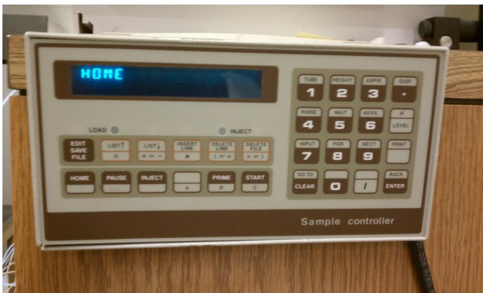
Figure B.7: Gilson Autosampler controller
